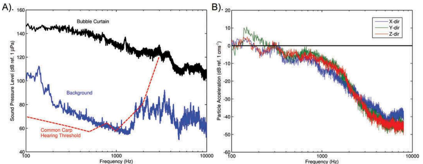
FIGURE 4. (A) Sound pressure level power spectrum of the bubble curtain (solid black line), background (solid gray line), and Common Carp hearing threshold (dashed red line; Popper 1972). (B) Particle acceleration in each direction: perpendicular (X-dir), parallel (Z-dir), and vertical (Y-dir) to the bubble curtain. Sound measurements were obtained 5 cm away from the bubble curtain in the center of the channel and 12.5 cm from the tank bottom.
