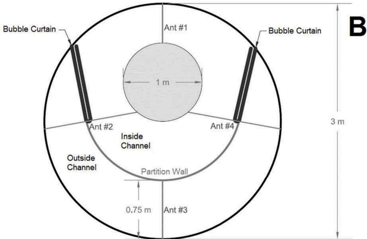
FIGURE 1. (A) Top view of the experimental bubble curtain tank. Bubble curtains (90 cm long white PVC pipes) are located at the end of the 50-cm-high partition wall. Water depth was 25 cm. (B) Overhead schematic of split-path circular channel showing position of bubble curtains and PIT antennas. Antenna number 3 was tuned and positioned to only detect movement through the outside channel.
